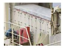
**Dust sealing system**Vibrating canevas
